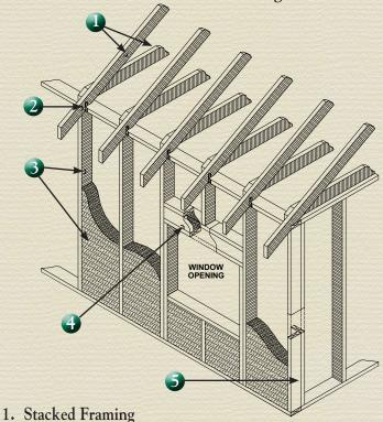
The components of the frame align on top of each other which efficiently transfers the load or weight down to the foundation, increasing the home's strength.
